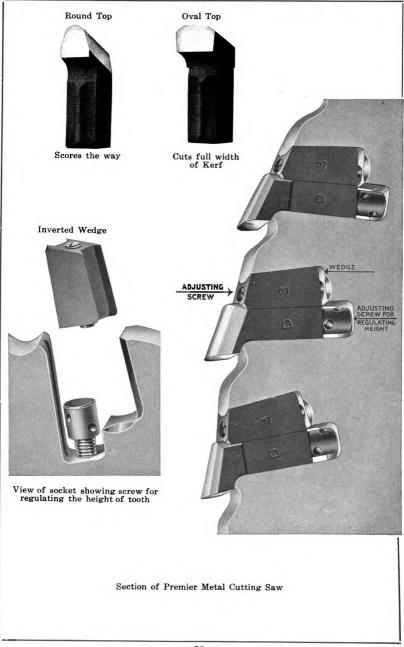
being made of High-speed Steel and weighing 1 pound; the wedge weighed  $\frac{1}{2}$  pound, thus making a total weight for the teeth and wedges alone of 84 pounds.
