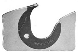
Concave Saws are employed in the manufacture of chair parts, for cutting the heads for barrels, kegs and bottoms for baskets. In fact, anything to be cut in rounded or curved form. This kind of work was done entirely by hand, or on Jig Saws, before the invention of the Concave Saw.
