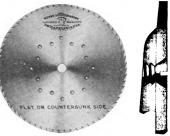
Shingle Saw and Method of Attaching it to Flange
