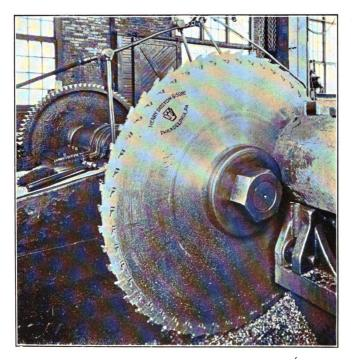
26-inch Blade, Bar Cold Saw Cutting Off Machine
